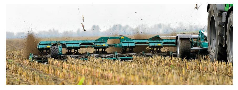
Thanks to its folding-swivel mechanism, the largest model of the NOMADE knife rollers achieves a transport width of 2.65 meters and an overall length of 7.55 meters.
