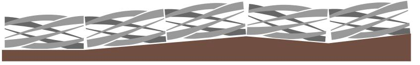
The INNOMADE knife rollers consist of approximately 1-meter-wide tandem knife units, each made up of two knife shafts operating in sequence. Thanks to the double-sprung coupling arm, the tandem knife units can move independently and adapt individually to the ground contours. This ensures consistent ground contact, optimal adaptation to terrain variations, and a uniform cutting patrern — even under changing and highly demanding conditions.
