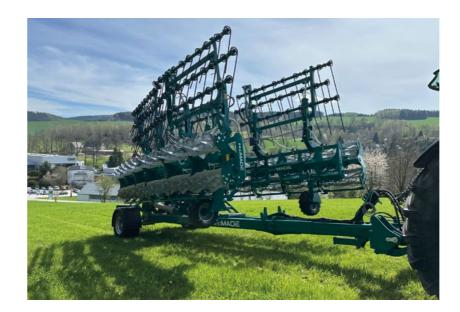
The MW1250 comes standard with a lower link hitch including hydraulic locking. This ensures safe stabilization of the knife roller during folding and unfolding – especially under negative tongue load.
