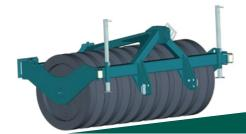
effective working width 280 cm o possible total weight (without additional equipment) 4.845 kg
