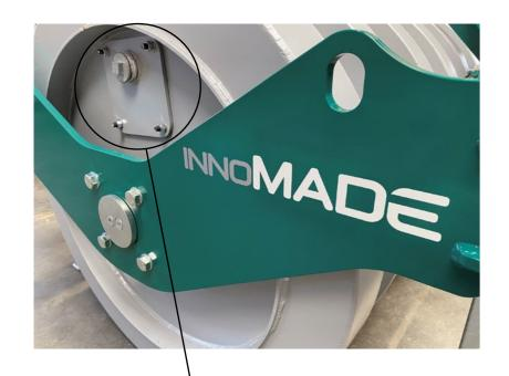
The INNOMADE Silage Roller can be filled with either water or sand via side openings. When filled with sand, the SW300 reaches a maximum total weight of 5,170 kg.
